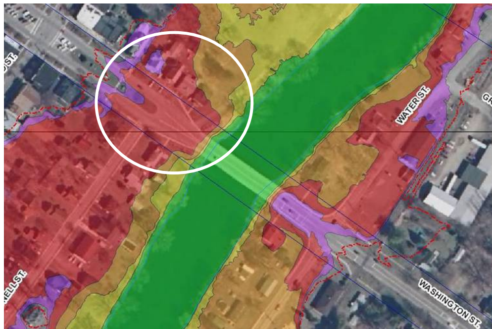
Figure 3: Inundation mapping demonstrating scenario #2. Notice that the bridge approach is blocked by floodwaters at moderate flood stage, yet the bridge deck is shown in green.
